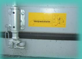
Photo is showing the security cam and cam keeper at locking rod No.3. It's also showing the chain door-holdback and door gasket. Holdback can also be made from nylon rope or similar.
