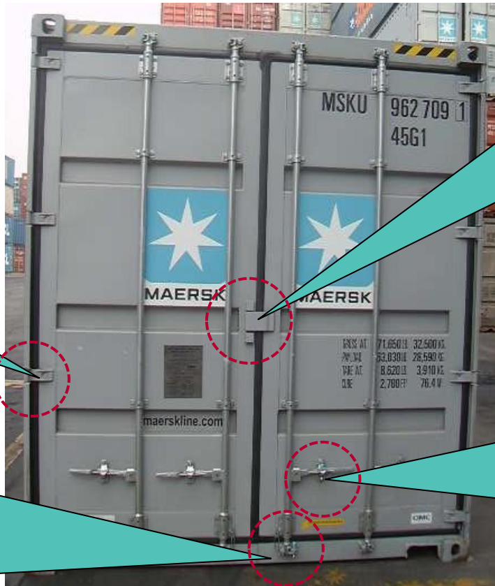
Door hinge components: Hinge pin, nylon bushing, hinge lug and hinge blade.
